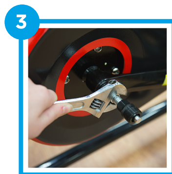
Insert the silver end of the crank remover and turn anticlockwise
